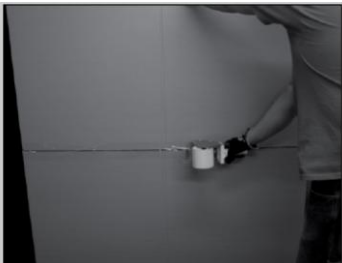
STEP #9-Tape Middle Seam of Half RSC Boxes
