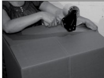
STEP #6- Tape Bottom of Half RSC Tubes
