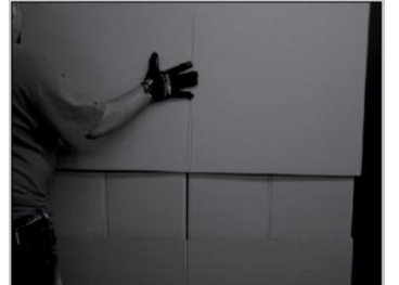
STEP #8- Slide Taped Half RSC Box over Top of Half RSC Tubes
