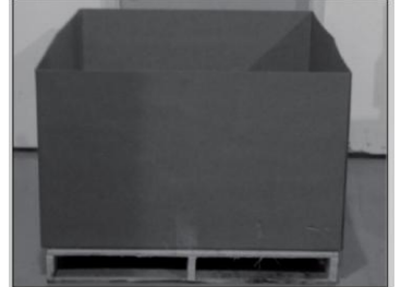
STEP #4- Place Half RSC Box on Pallet
