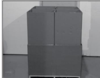
STEP #7- Insert All Half RSC Tubes into Palletized Half RSC Box
