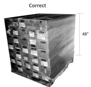
Correct 48” High Properly Stacked Ends Sealed No Lamp Exposed Shrink-wrapped
